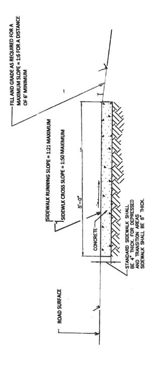
CONCRETE SIDEWALK DETAIL NO SCALE
